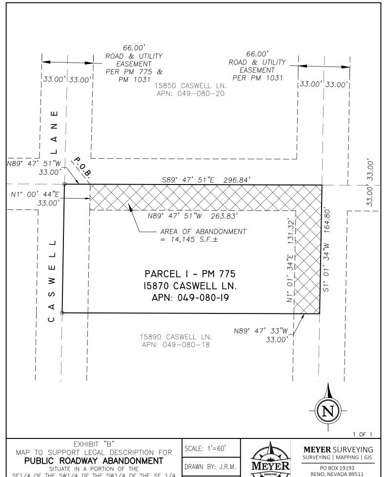
SE1/4 OF THE SW1/4 OF THE SW1/4 OF THE SE 1/4 OF SEC.34, T.18N., R.19E., M.D.M WASHOE COUNTY, NEVADA
