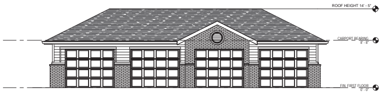
1 GARAGE FRONT ELEVATION - 4 BAY STANDARD 3/16" = 1'-0"
