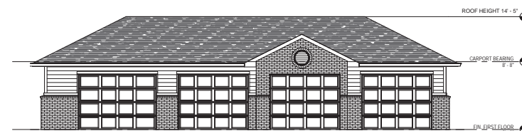
1 GARAGE FRONT ELEVATION - 4 BAY HC 3/16" = 1'-0"
