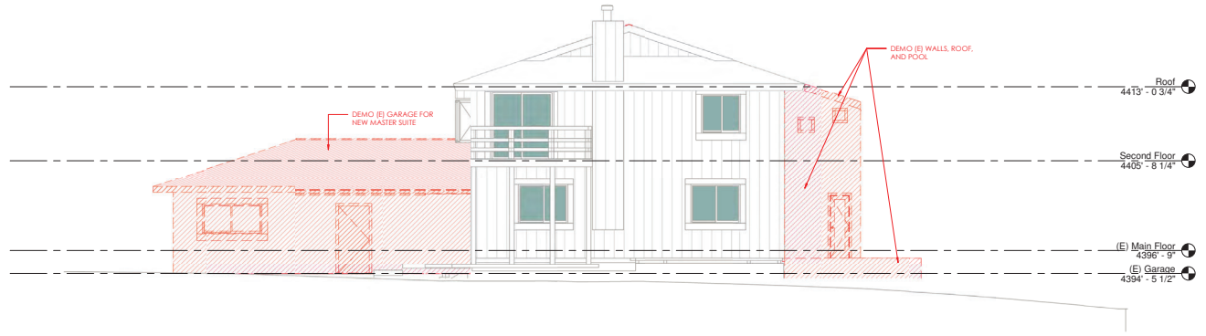
1 West Elevation - Existing Demo 3/16" = 1'-0"
