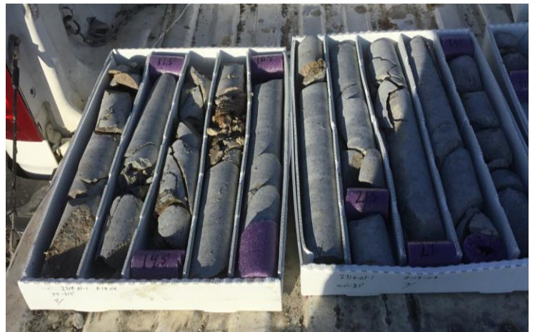
Photo of Rock Cores in B-19-09 at 7.5' to 31.5' Depth Showing Widespread Competent Granitic Bedrock
